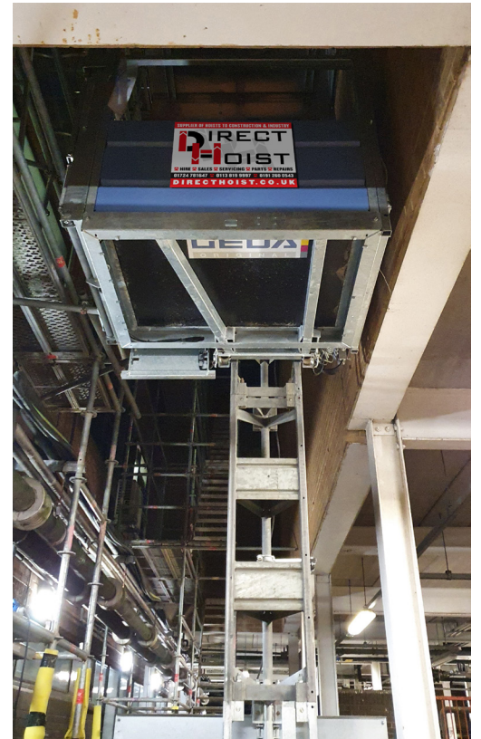
On hire from Direct Hoist, this GEDA 300Z ZP can lift 300kg or three people in personnel mode.
